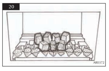
6.17 Place three small coals at each end of the front coal so that they lean against the flame baffle and a further four large coals on the flame baffle, two at each end, see diagram 21.
